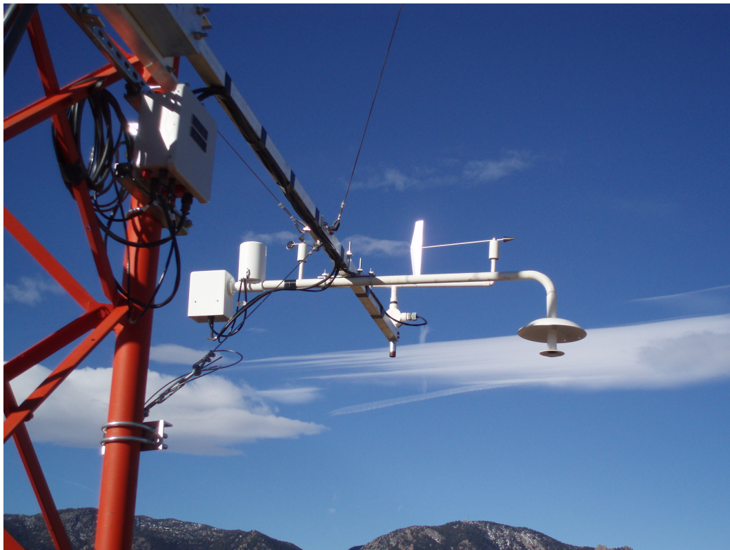
Figure 11. Co-located wind sensor WS-201 and aspirated thermal radiation shield M0327C at 3 m above ground on the M4 mast. Author's own photograph.
